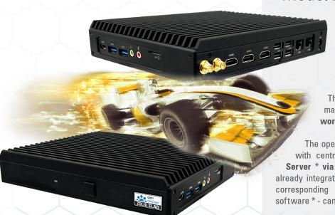
The ZOLID.SLAB is powered by an Intel® Celeron® processor, providing powerful performance for demanding applications. Additionally, it features three HDMI 2.0 interfaces, allowing for easy and fast use with multiple displays.
